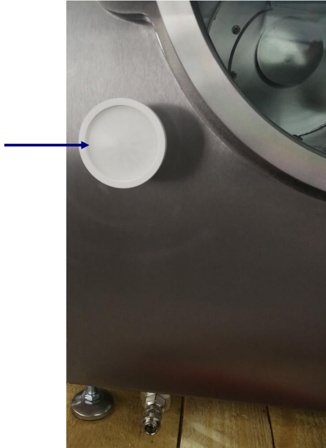
Figure : Venting air filter of Laboklav 25
