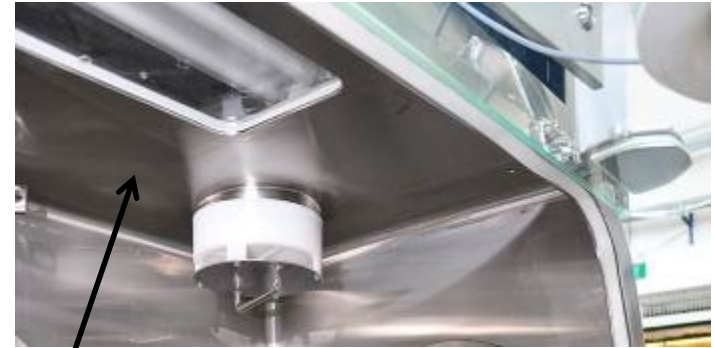
2° Sloped ceiling to the rear to reduce water droplet retention after WIP/CIP
