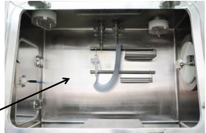
2° Sloped ceiling to the rear to reduce water droplet retention after WIP/CIP
