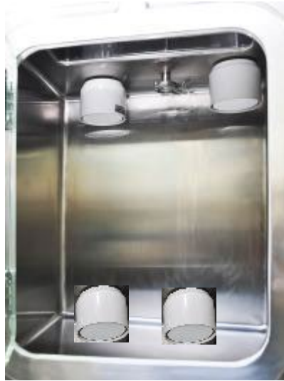
Pass In the New Clean Filters & Close the Outer Pass Chamber Door
