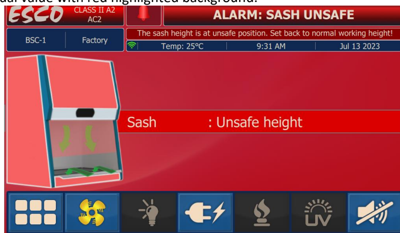
Figure 14. Alarm Unsafe Sash Height
