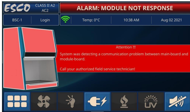
Figure 15. Alarm Module Not Response
