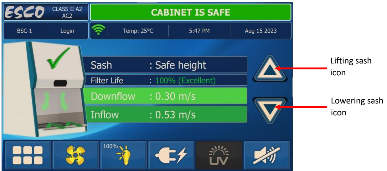
Figure 9. Main Screen Display for Motorized Sash
