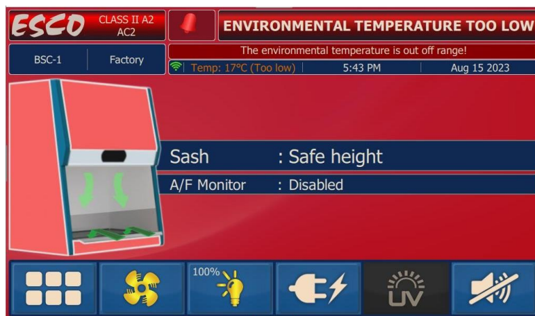
Figure 17. Ambient Temperature is Too Low
