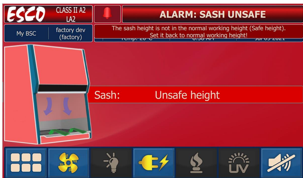
Figure 13. Alarm Unsafe Sash Height
