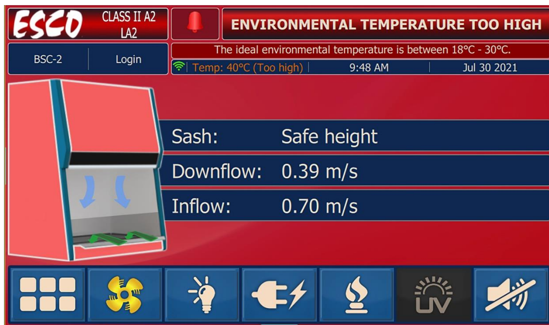
Figure 17. Ambient Temperature is Too High
