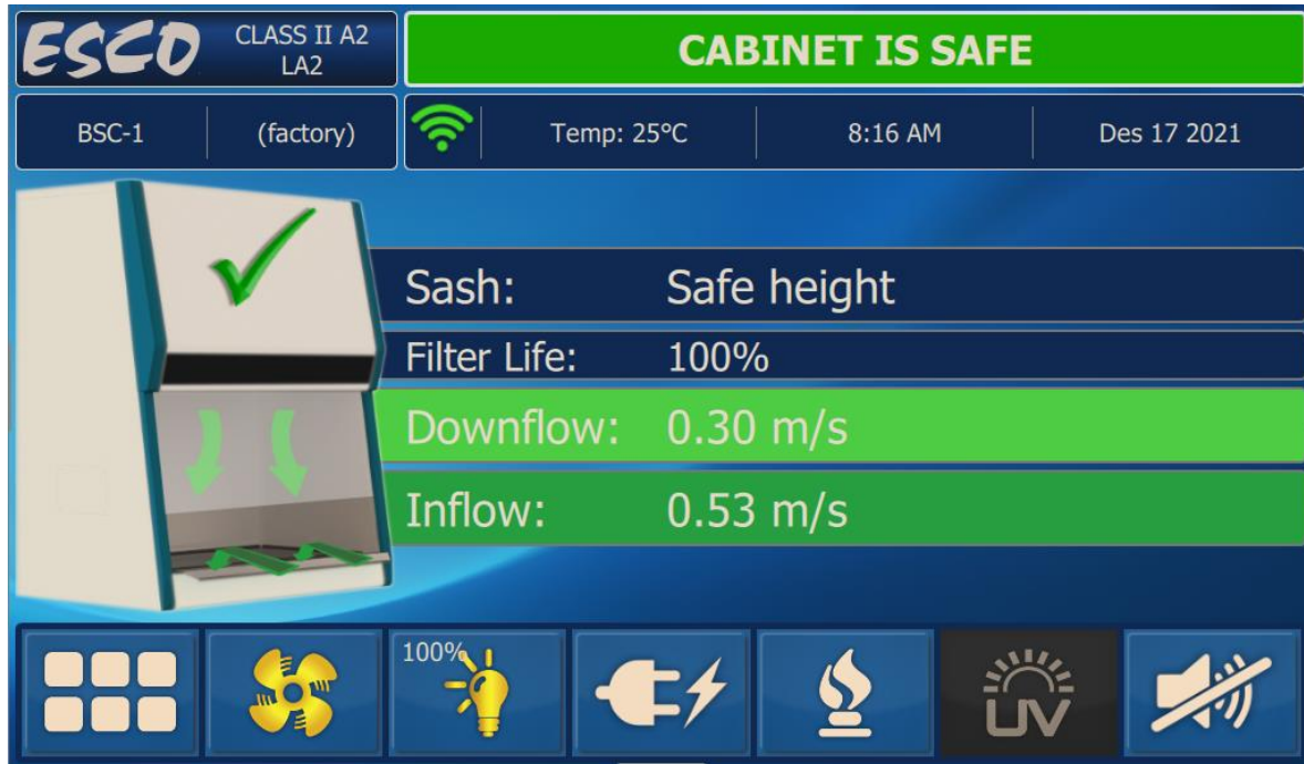
Figure 11. Operational Safe Condition
