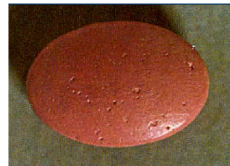
Dissolution of stearic acid caused pitting 2
